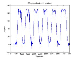
Figure 4: Noisy Rotation angle calculated by the Accelerometer
