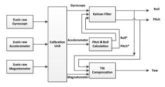
Figure 5:System Structure
